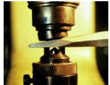
Special tool control for blade hardness.
