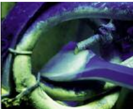
Checking for hairline cracks.
